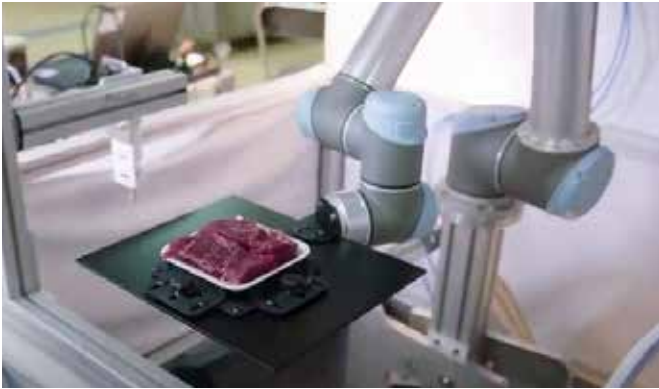
The robot loaded and ready for sampling. Future meat quality assessment could be done in real-time in the plant, using a robot like this, guaranteeing consumers a high-quality experience.
